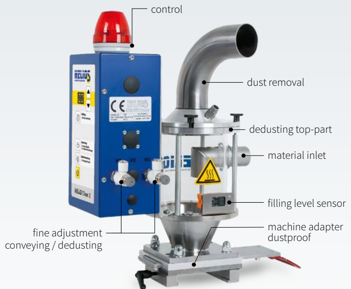
Example: HELIO®Clean 2, compact version, 1 component
