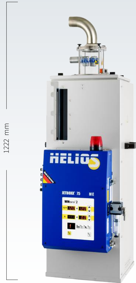
JETBOXX®-Set 75 liters Example: + 2c-conveyor with exhaust air filter Throughput : 10 – 15kg|h
