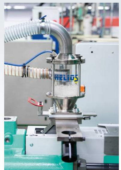
HELIO®Clean 2 on processing machine. Control version CE included as second conveying point in JETBOXX® dryer
