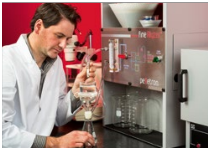
FineAlyzer®, Pelletron Corporation's wet test device
