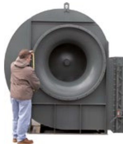
Fan for iron ore cleaning
